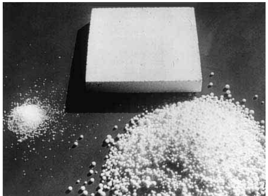
Fig. 6 The processing stages in the production of EPS foam: raw material (left), pre-expanded particles, moulded foam.
