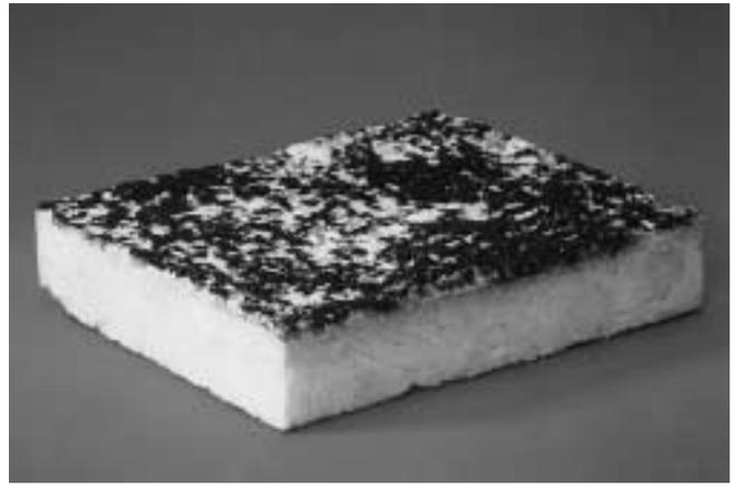
Fig. 2 Specimen taken from flat roof as shown in Fig. 1. No changes can be discerned in the Styropor.
