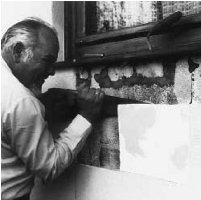
Fig. 3 Taking a sample of Styropor from an outdoor composite insulating system consisting of Styropor and a fabric-reinforced textured finish.
